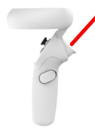
Trigger Button is on underside of controller.
